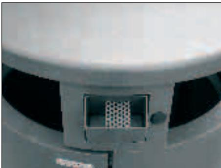
The CIGAFOX litter bin is made from a cylindrical structure which includes a fixed semicircular back in 10/10mm thick galvanised sheet steel, a semicircular door in 10/10 galvanised sheet steel and a galvanised sheet steel cover, fixed to the structure with stainless steel fixings. Incorporated within the supports that hold
